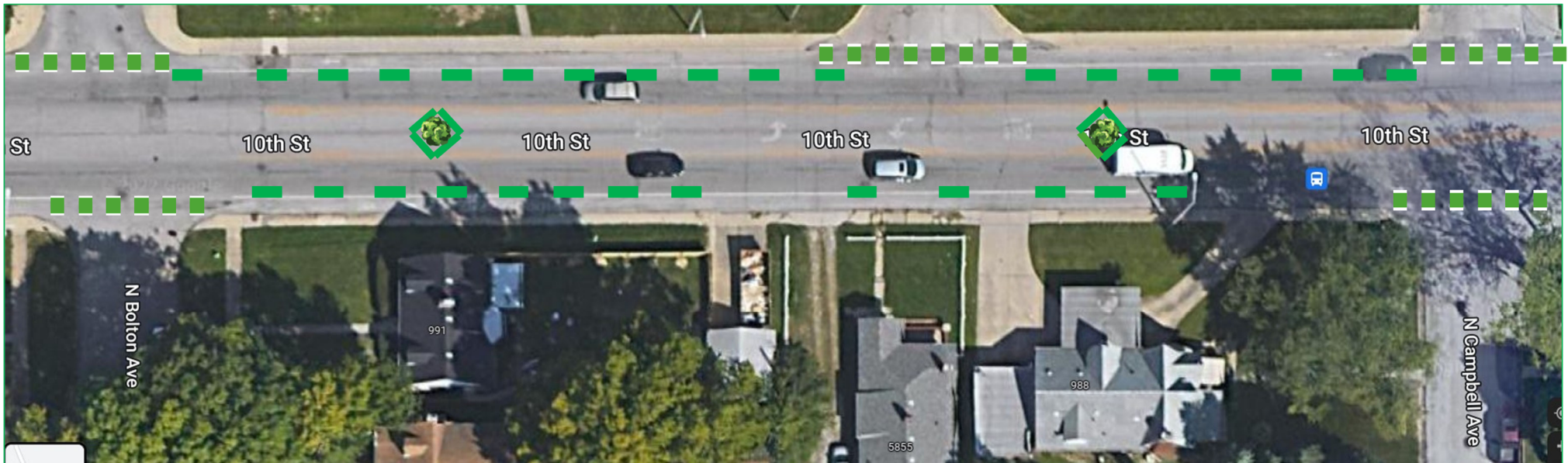
Figure 94. Detailed design plan of the bike lane green paint, a diamond pattern water walls with street tree, and the bike lane water walls on 10 th St. between Bolton and Campbell Ave.
