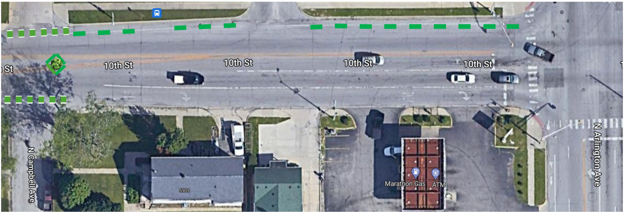
Figure 95. Detailed design plan of the bike lane green paint, a diamond pattern water walls with street tree, and the bike lane water walls on 10 th St. between Campbell Ave and Arlington Ave.
