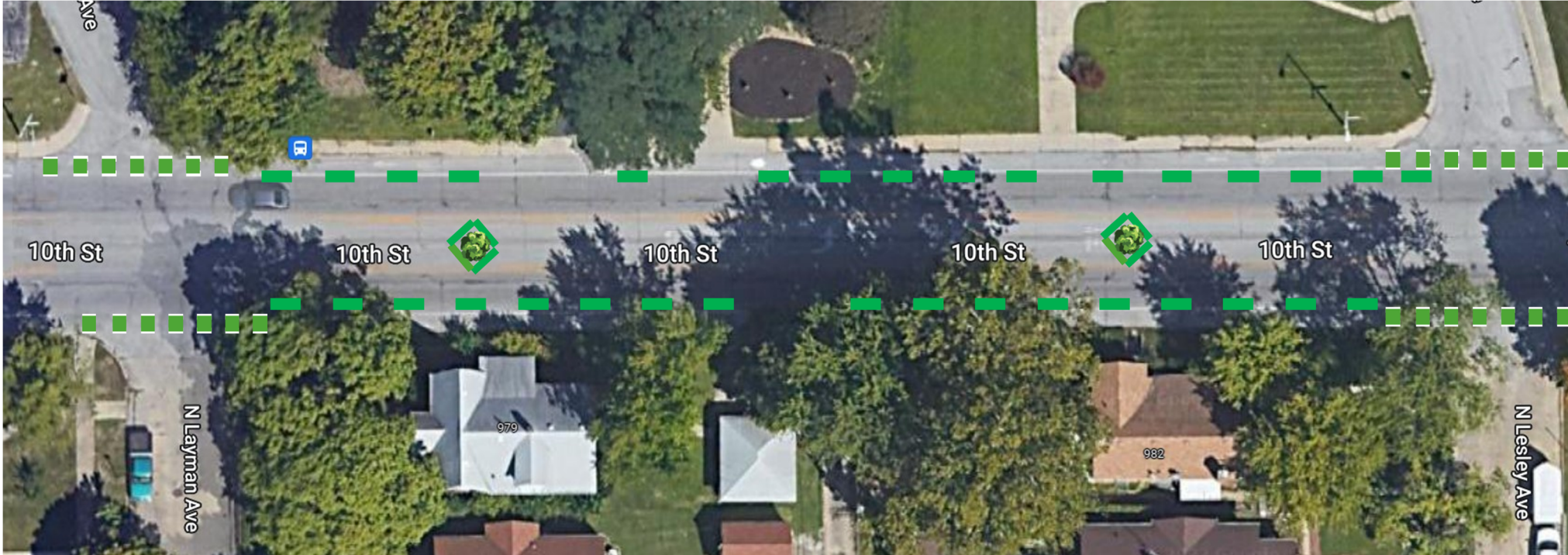
Figure 90. Detailed design plan of the bike lane green paint, a diamond pattern water walls with street tree, and the bike lane water walls on 10 th St. between Layman Ave and Lesley Ave.
