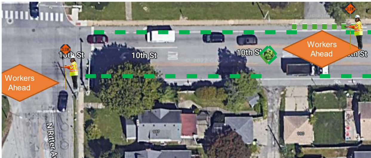
Figure 99. To install the bike lane water walls, two “WORKERS AHEAD” signs, and two volunteers with “SLOW” signs will be used to notify drivers of ongoing work.
