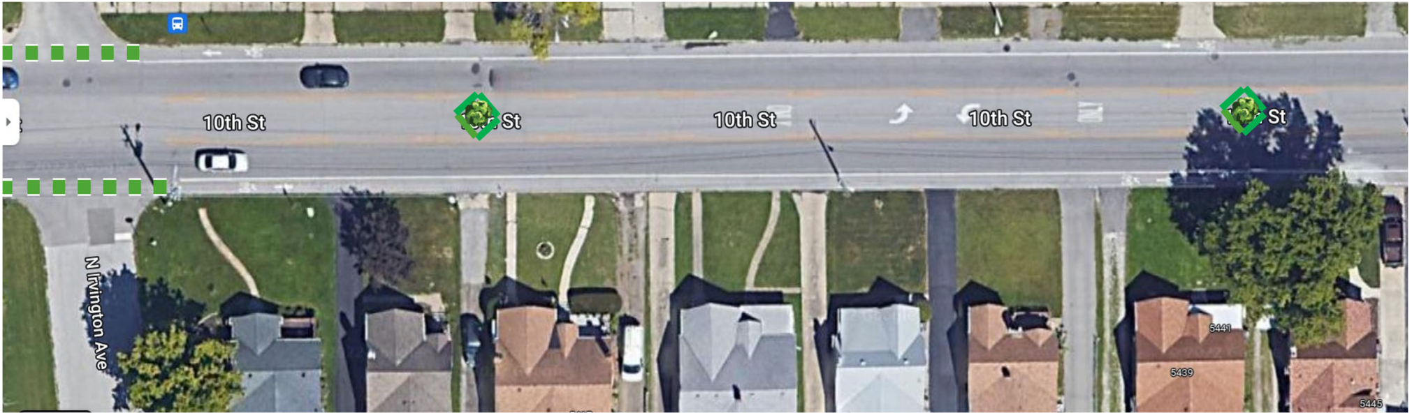
Figure 87. Detailed design plan of the bike lane green paint and two diamond pattern water walls with street trees on 10 th St. between Irvington Ave and Ellenberger Pkwy W Dr.
