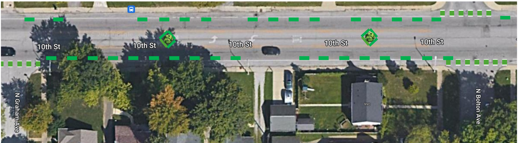
Figure 93. Detailed design plan of the bike lane green paint, a diamond pattern water walls with street tree, and the bike lane water walls on 10 th St. between Graham and Bolton Ave.
