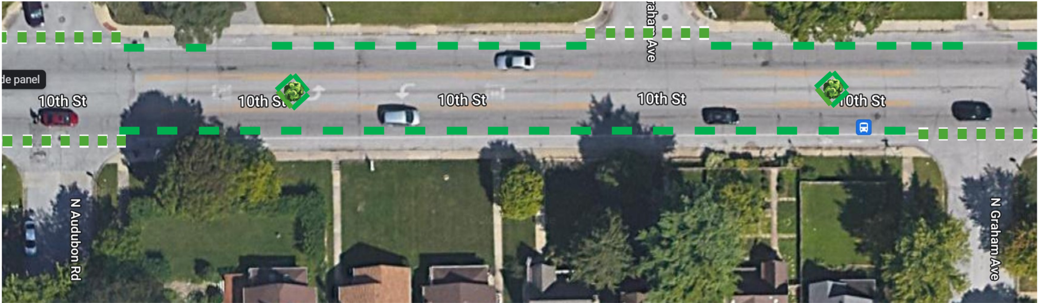
Figure 92. Detailed design plan of the bike lane green paint, a diamond pattern water walls with street tree, and the bike lane water walls on 10 th St. between Audubon Rd and Graham Ave.
