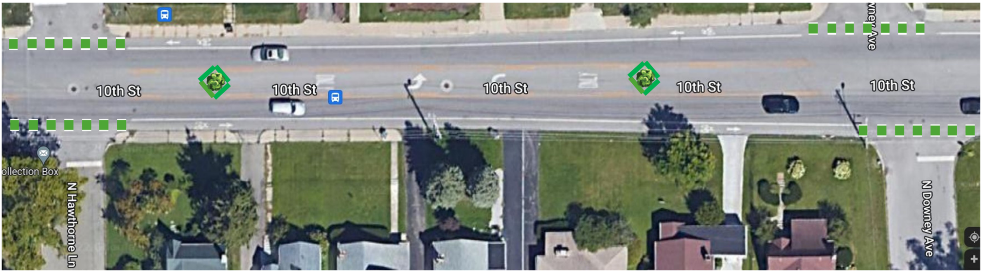
Figure 85. Detailed design plan of the bike lane green paint and two diamond pattern water walls with street trees on 10 th St. between Hawthorne Ln and Downey Ave.
