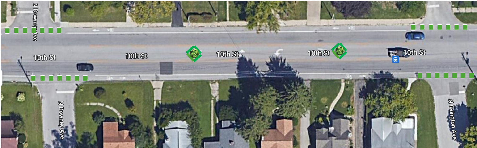
Figure 86. Detailed design plan of the bike lane green paint and two diamond pattern water walls with street trees on 10 th St. between Downey Ave and Irvington Ave.
