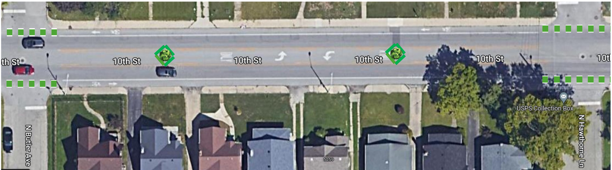
Figure 84. Detailed design plan of the bike lane green paint and two diamond pattern water walls with street trees on 10 th St. between Butler Ave and Hawthorne Ln.
